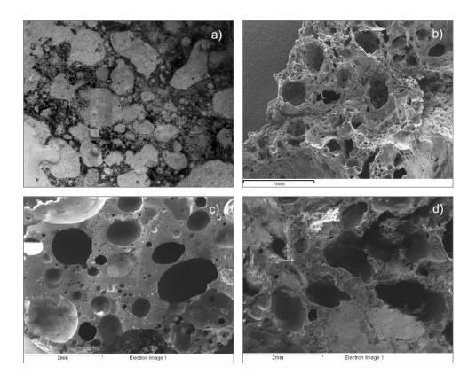
**Figure 2** shows the highly porous nature of P166/100 and M224/100. (a) Thin section montage of P166/100 in plane polarised light. Voids show up in light grey (resin pores) with K-rich glass in dark grey/black. (b) SEM (GSE) of P166/001 showing extensive voids. (c) SEM (BSE) of M224/001 (polished) and (d) SEM (GSE) of M224/001 using the FEI (Phillips) XL30 FEG at the School of Earth and Ocean Sciences at Cardiff University.
