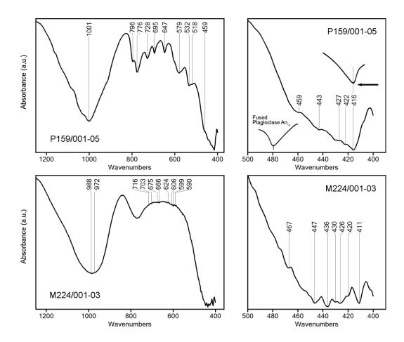
**Figure 4:** Shows FTIR spectra for samples P159/001-05 and M224/001-03. The degradation of spectral features in the 480 cm<sup>-1</sup> to 580 cm<sup>-1</sup> region can be seen in M224/001-03. The band at 459 cm<sup>-1</sup> corresponds to the Si-O asymmetrical band of vibration. Note the absence of a band at 780 cm<sup>-1</sup> due to vibrations in tetrahedral site symmetry (Schneider<sup>25</sup>, 1974; Parthasarathy et al.<sup>24</sup>, 2001, Saika et al.<sup>26</sup>, 2007).
